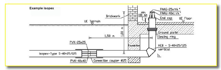
House-entry-elbows are useful for connecting buildings without cellars by passing the concrete ground-plate of the house. They will be produced generally in standard lengths of 1,00 x 1,50 m. Depending from kind of flexible pipe with steel, copper, PE-Xa or PE100-carrier pipe. For post insulation of the connection spot in the soil a jacket pipe connecting coupler will be required, see Design-Manual, chapter 6.
