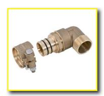
Orders for alignment-angles should bear the exact description and operating pressure. The connection to the isopex pipe end is carried out as a screw or clamp connection, whereby the screw connections are only used at accessible material transitions in buildings or shafts.
