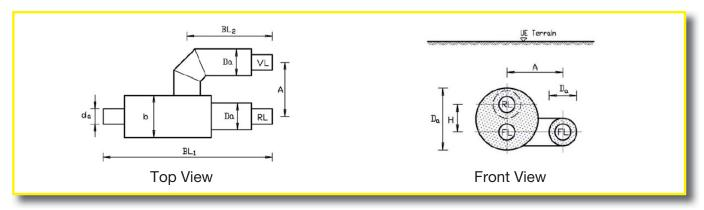
Bifurcated pipes are used for transition of two single pipes to one double pipe and are produced generally with the same dimensions. For **isoflex**-applications, bifurcated pipes will consist of steel carrier pipe, for **isopex**-Heating and **isopex**-Sanitary of crosslinked PE-Xa. In relation with **isocu** they will consist of copper pipes according to DIN 1754/17671.
